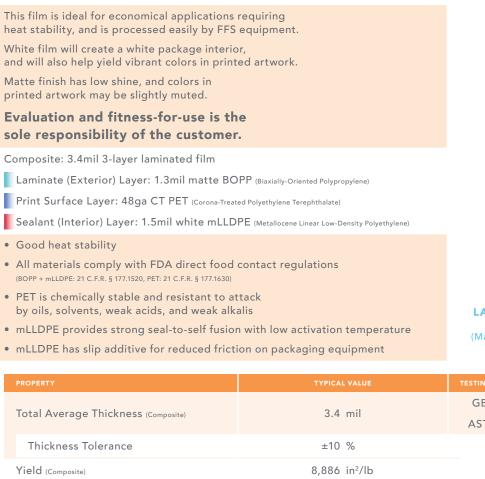
LAMINATE PRINT SEALANT LAYER LAYER LAYER (Matte BOPP) (CT PET)
